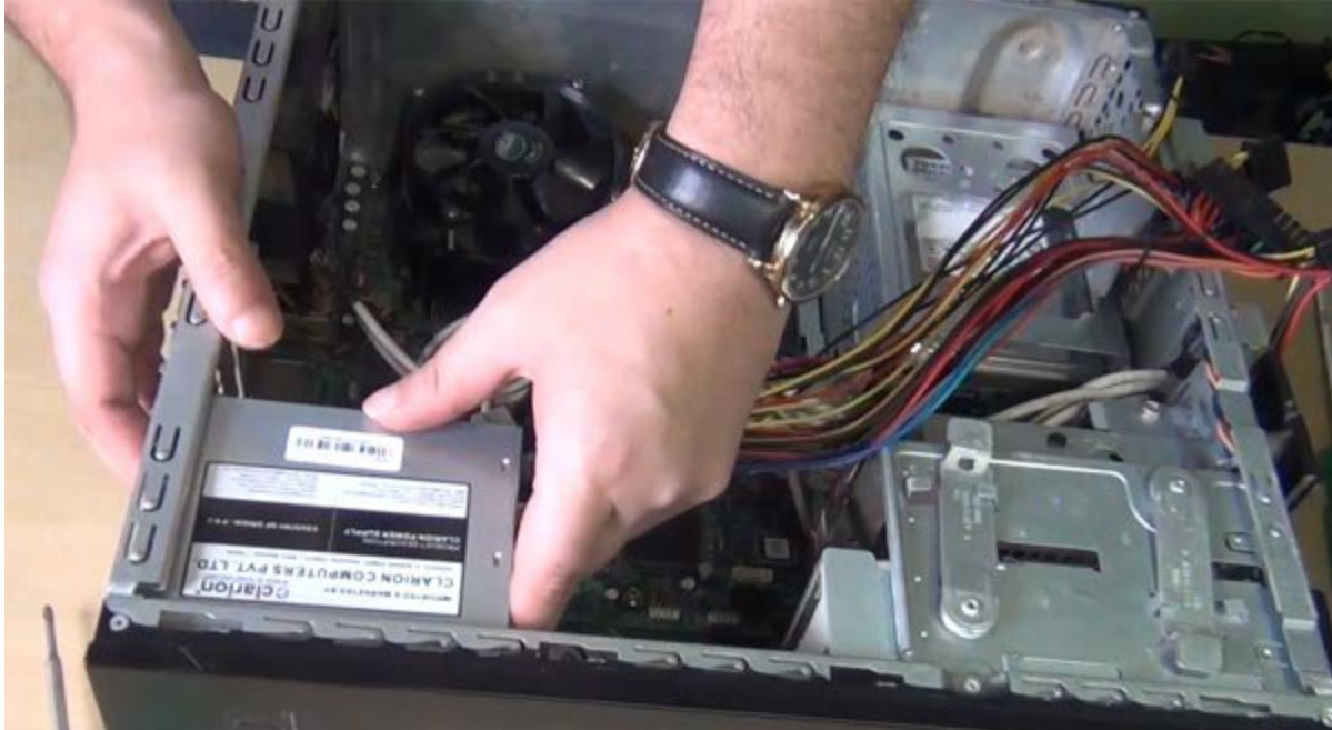
Fig: Install Power supply unit (SMPS)
