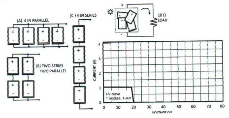
Draw the I-V curves for all three combinations on the same graph. Which wiring system would be best?
